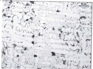
Fig. 1: Microstructure of Cast Iron
